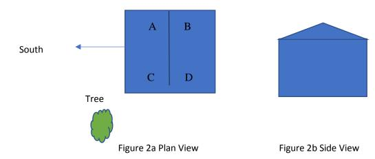
Figure 2 is the roof of a house, and the roof has a pitch to the center of 15 degrees. The system will consist of 2 modules mounted on top. There is a tree that will shade the south-east section of the roof. The latitude is 20 degrees north. On what section of the roof (A, B, C or D) should the modules be installed?
