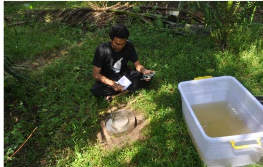
Measuring infiltration rate
