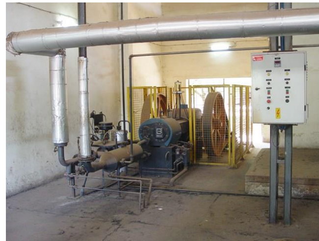
60 kWe Steam engine run on cashew shell at SICAJU in Guinea Bissau
