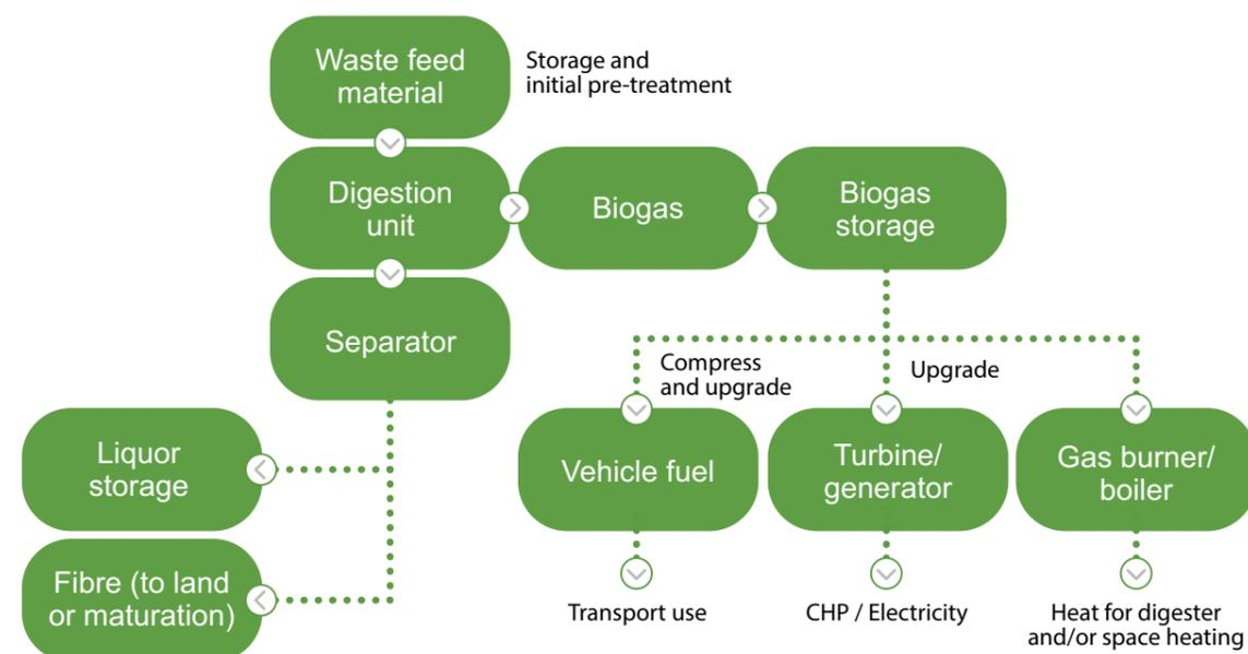
Additionally, before biogas can be converted into electricity in turbines, the raw biogas must be desulfurized and have moisture exacted<sup>10</sup> (Figure 13). These summarise only a small set of the variables that a biogas plant designer must take into account, necessitating expert input for even relatively basic design decisions and estimates of feasibility.
