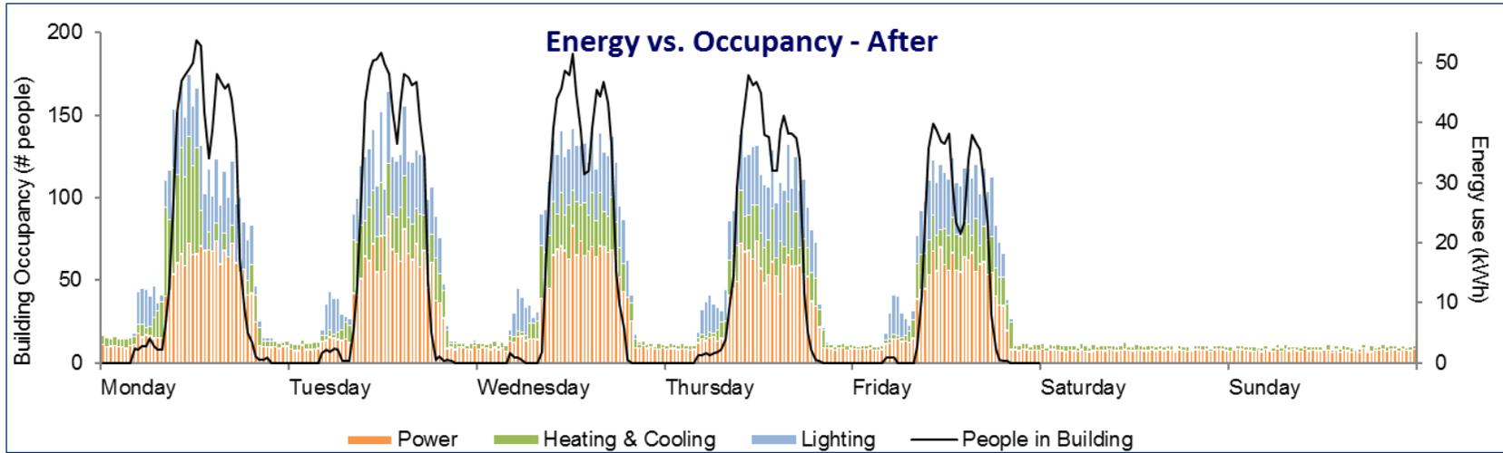
Large cost savings by removing most of the baseload consumption!
